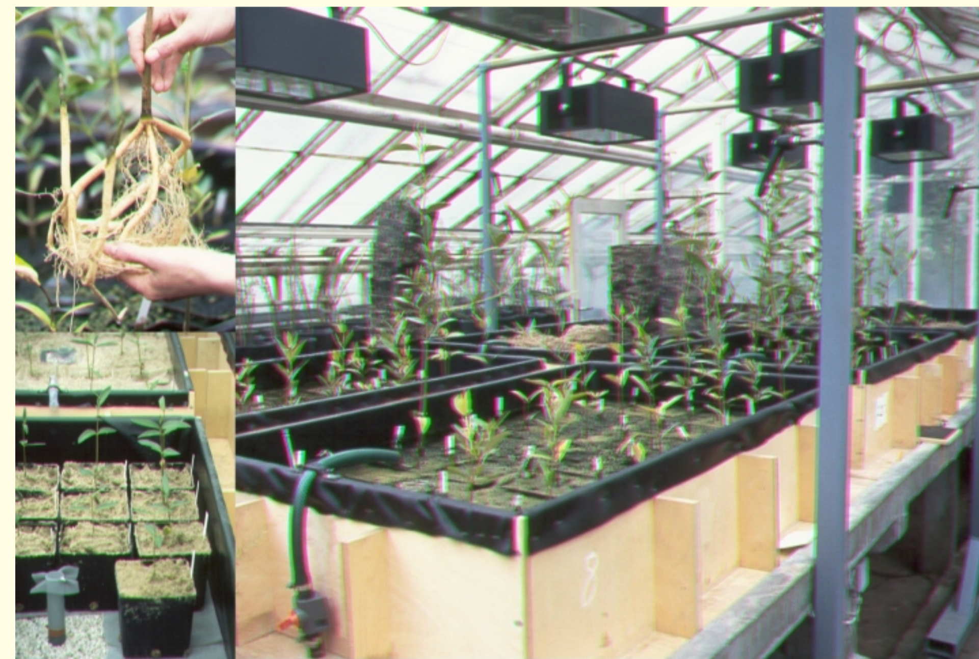
Fig. 1: Growing of Avicennia marina in plant breeding boxes with simulation of tides. Small picture on the top: roots of A. marina , small picture at the bottom: plant breeding box at the installation.
